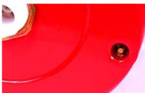
Bleed valve for rapid depressurisation and aut drain function check.
