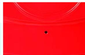
Pressure relief hole gives an audible warning if any attempt is made to remove filter bowl whilst under pressure.
