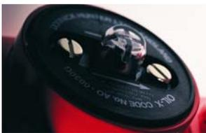
Differential pressure monitor fitted as standard on filters 3/4" and larger. (except AC/ACS/AX grades).
