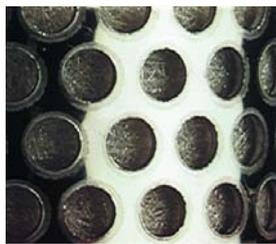
**Stainless steel inner and outer support cylinders**
