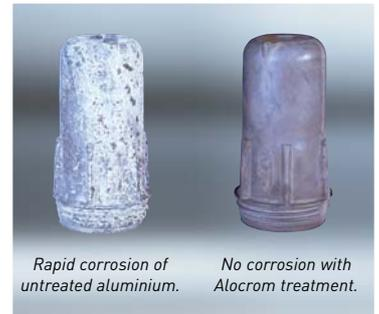
Rapid corrosion of untreated aluminium.
